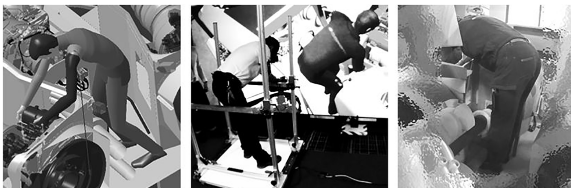
Figure 6. The operator performing a maintenance task with similar ergonomic characteristics for digital human modeling, the virtual reality platform, and the physical mock-up.
